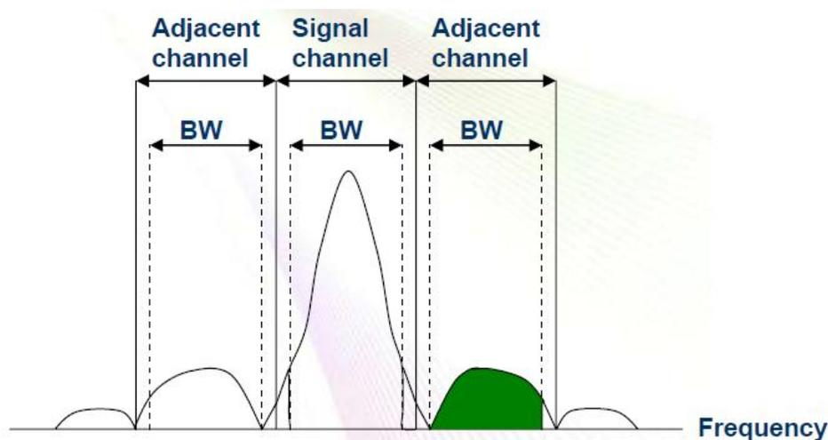
Figure 2. Signal bandwidth and adjacent channel transmit power
