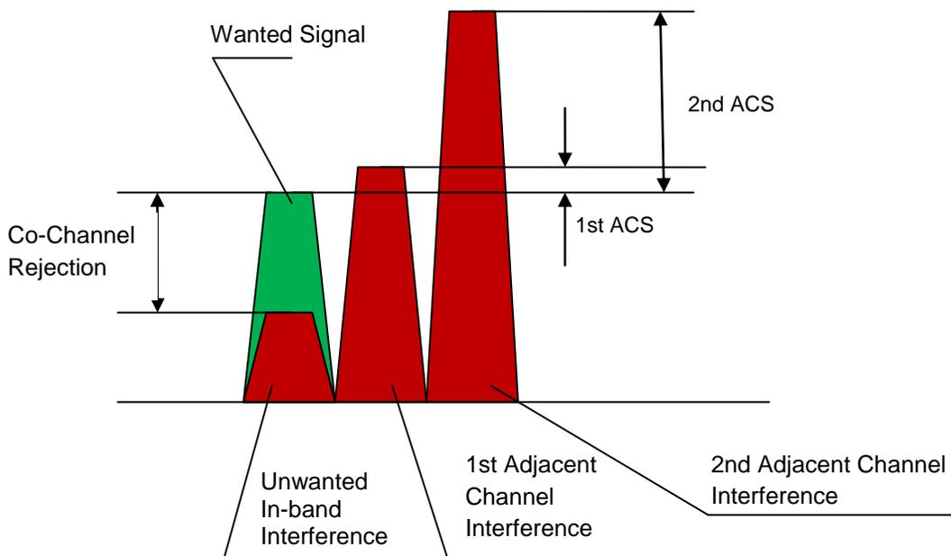
Figure 3. Co-Channel Rejection and Adjacent Channel Interference
