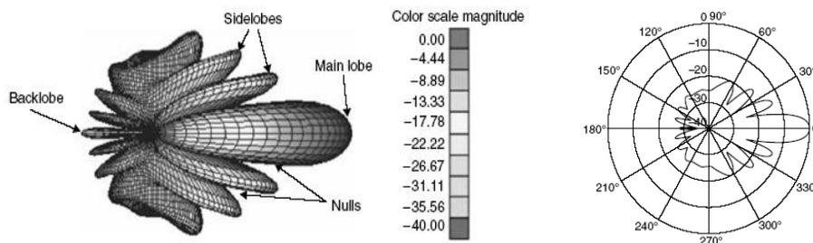
Figure 1: 3D radiation Pattern and the Polar plot of a complex antenna
