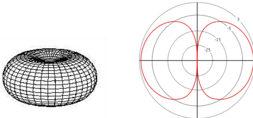
Figure 2: the 3D Radiation Pattern and the gain (in dBi) of a half-wave dipole, A dipole has 2.15dBi gain.
